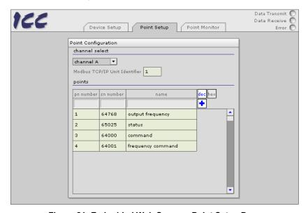
Figure 21: Embedded Web Server – Point Setup Page
